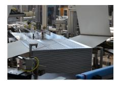
The Vapobloc is assembled in the same way as the classic POLYBLOC plate heat exchanger. The distance plates are made out of corrugated aluminium plates which gives the plate heat exchanger its unique mechanical stability.
