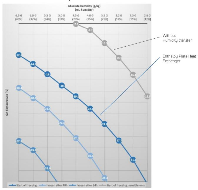
Start of Freezing: At this temperature the maximum relative humidity of the leaving air (100%) is reached. Below this temperature there will be some condensate
