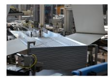
The Vapobloc is assembled in the same way as the classic POLYBLOC plate heat exchanger. The distance plates are made out of corrugated aluminium plates which gives the plate heat exchanger its unique mechanical stability.
