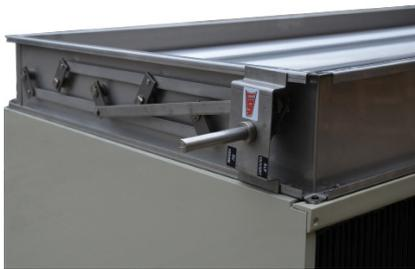
Block casing made from 20 mm polypropylene plates, with plastic composite corner profiles. These are reinforced with fully encapsulated stainless steel profiles. With integral bypass enclosure and aluminium bypass damper. Bypass damper also available on request in stainless steel or plastic.
